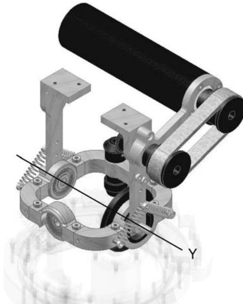
Fig. 19. A detailed view of the nod mechanism. The blue part can rotate relatively from the red part around the Y -axis.
