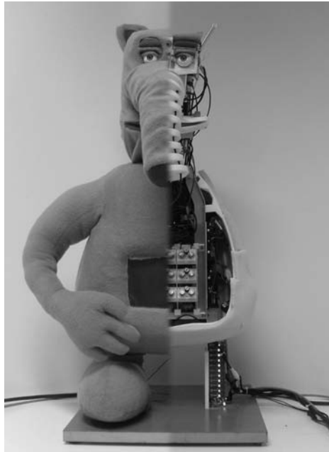
Fig. 5. A section view of the real Probo prototype.
