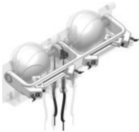
Fig. 7. The backside of the system. The rods to pan the eyes are highlighted in blue.
