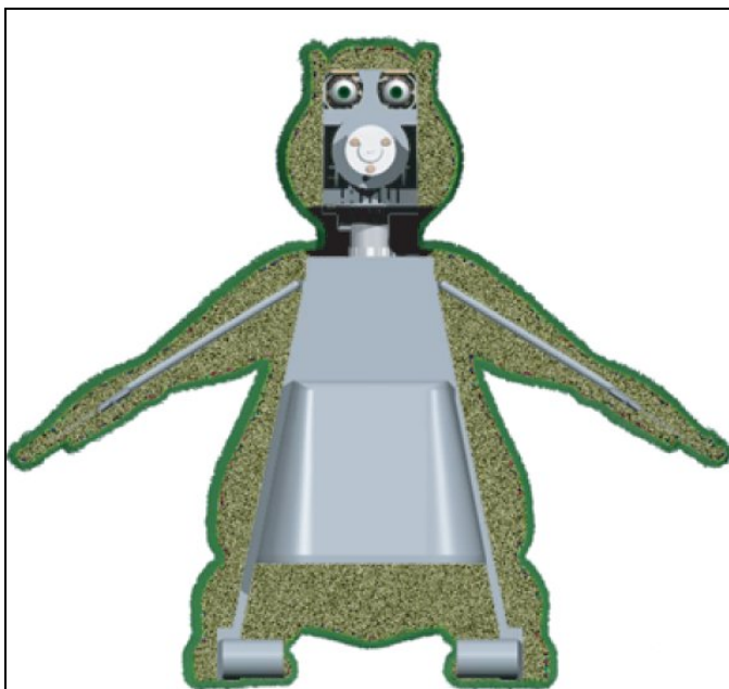
Fig. 6. Section view. The fur and foam protect the internal robot.
