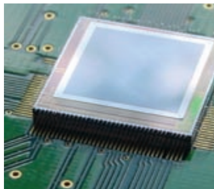
35µm-backside-thinned APS image sensor on a readout chip, wirebonded to a test board.
